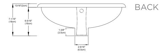
By IAPMO, ceramic lavatory warpage is defective only if warpage of flat slab out of horizontal plane exceeds 6.3 mm/m (0.25 in/ft) on all sizes OR warpage on back of lavatories that are attached to the wall exceeds 3 mm (0.13 in).
